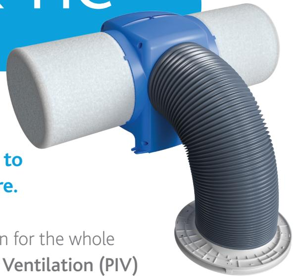
The **DRI-ECO-LINK-HC** offers a ventilation solution for the whole property, using the tried and tested **Positive Input Ventilation (PIV)** principle, where fresh, filtered air is introduced into the home at a continuous rate, encouraging movement of air from inside to outside.
